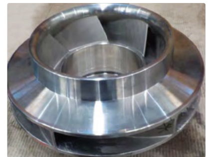
Feed pump water jackets and feed pump impeller
