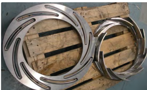
Machined & fabricated diffuser, replacing a failed cast diffuser
